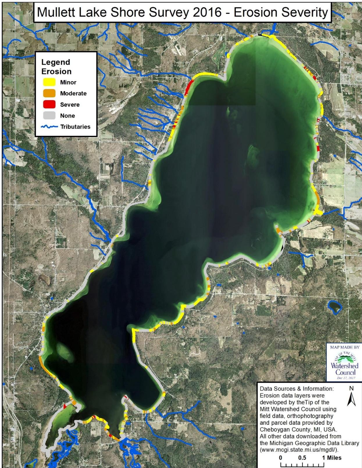
Figure 7. Shoreline erosion severity results for Mullett Lake
