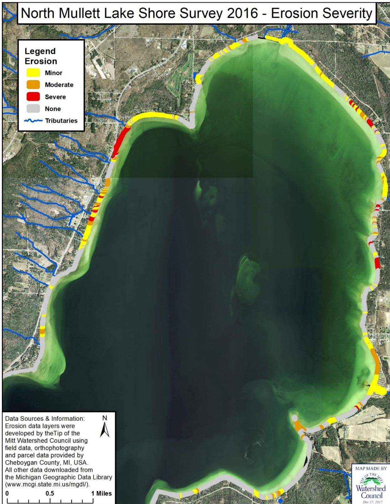
Figure 9. Northern shore Mullett Lake erosion severity
