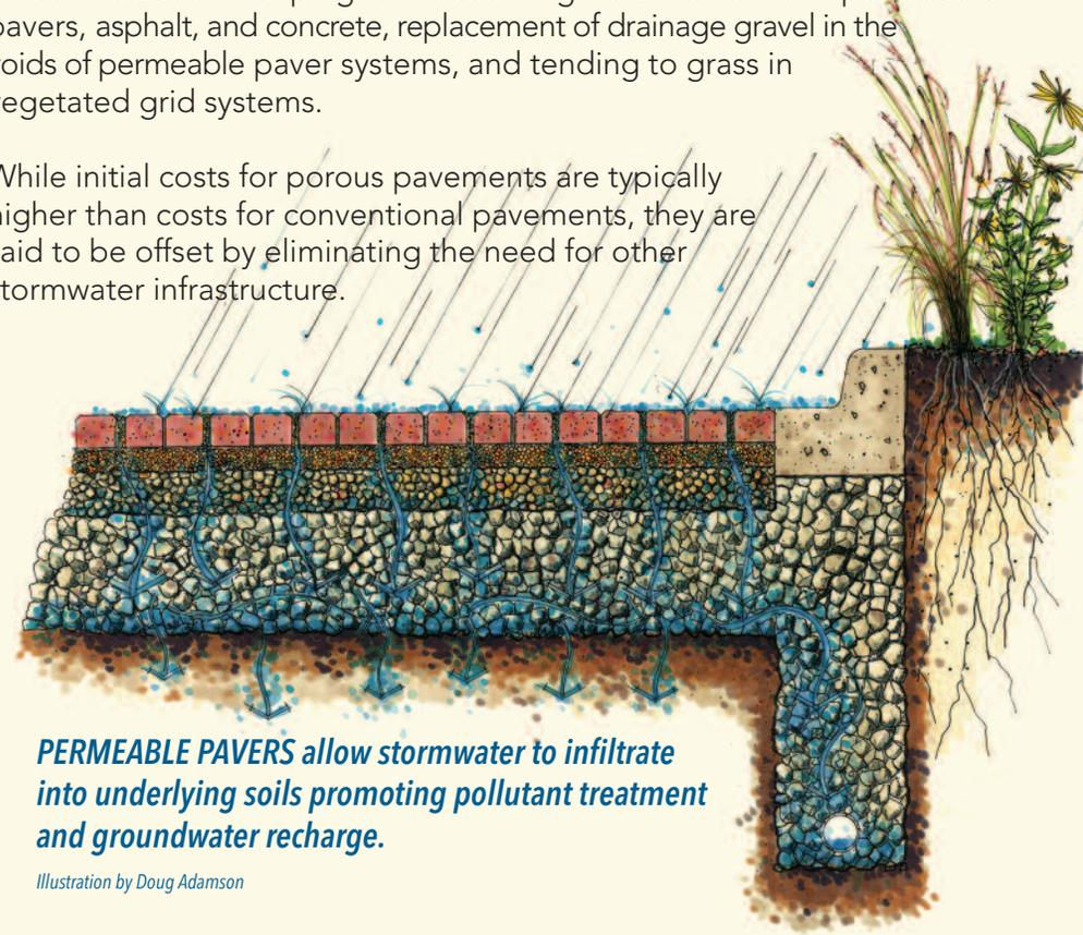
**PERMEABLE PAVERS** allow stormwater to infiltrate into underlying soils promoting pollutant treatment and groundwater recharge.
